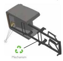
E: Next, pull away the dust cover which is attached with Velco® to the inside lower portion of the back section. This will provide access to the eight bolts attaching the Back Frame to the two Side Frames. Using a 1/2" wrench, or ratchet with socket, remove these bolts. Next, pull away the Velco® flap between the Back Frame and the Back, and place the Back Frame to one side.
